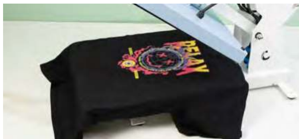
Vertical Heating Platen Ideal for T-shirt printing
